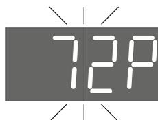
To set the limit temperature, press any button. It will be displayed and start to blink the set air temperature in the premises 'C'. As long as the value is flashing at the same time press and hold both buttons for at least 2 seconds. After the beep, it is displayed and starts flashing the set limit of the surface temperature of the heater 'P'. Set the new value and wait for 6 seconds to exit from the setting mode.
