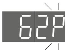
**Attention!** If the surface temperature of the heater is showed continuously, then the remote sensor is not connected (damaged). Irrespective of the room temperature the heater surface will be warmed continuously to the set value "P" (see below).
