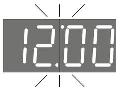
✳ To change the program cycle from daily to weekly week and vice versa ,in the time setting mode (see p. ❸), simultaneously press and hold both buttons, then no later than in 1.5 seconds take out and reinsert the plug into the socket and only after the appearance of the corresponding indication release the button.
